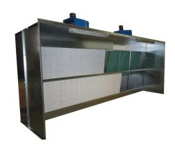
WFP dry painting booths in wall-mounted execution, are equipped with integrated filters and aspirator and thanks to their geometry form a suction front at constant speed so as to capture the exhalations produced by operations such as painting, resin coating, gluing and in all those professional treatments that generate non-dusty exhalations and overspray.
