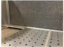
Anti-rebound suction front wall for grinding on SBA, SBF and SBV benches.
