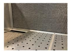
Anti-rebound front wall for SBC benches, consisting of a suction metal mesh net placed on the front of the bench for operator protection from splinters and sparks from high-speed grinding.
