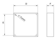
Rectangular spacer for fixing on thin walls for SEQ model fans.
