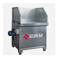
The SBV suction bench is designed to protect the operator from fumes and volatile dust emitted by professional processes such as welding, deburring, sanding or grinding of metals in the metalworking industry, foundries and all sectors where surface treatments with dry abrasives are carried out. It is also used for cleaning workpieces or blowing parts with associated dust emission.
