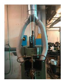
Light grey **flexible hose** made of robust **PVC**, helically spiralised, thanks to the material and construction it remains in a self-supporting 'suspended' position, a unique and very useful feature in the end sections of suction systems, as for example in the picture below taken from a pointing fume suction application.
