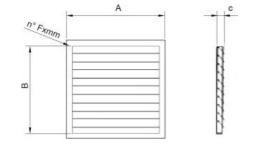
The SEQ axial fan gravity damper prevents heat loss when the fan is stopped, rain, wind and bird entry.
