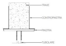
Fixing kit for SMHS fans in HVLS version compatible with rectangular section beams with base between 100mm and 260mm.
