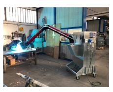
The DFC mobile wheeled fume and dust extractor is designed for the extraction and filtration of even very fine and volatile fumes and micro-dust generated during surface treatment processes of metals or composite materials.
