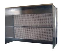
WFPE suction walls are designed to be connected to a suction system with an external fan. They are equipped with dry filtration and due to their geometry form a constant velocity suction front so as to capture pollutants produced by operations such as painting, resin coating and bonding.
